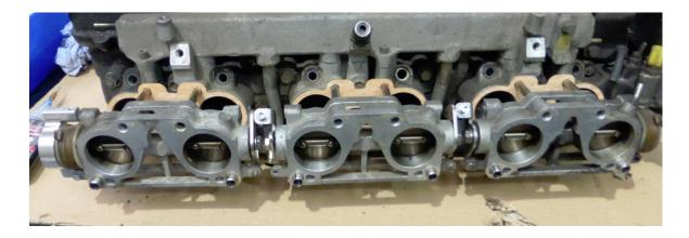
Fit the first set of new gaskets and slide on the 3 throttle chambers. Push all 3 chambers against the head.
