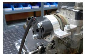
Attach the TPS supplied using 2 x M4 screws and flat washers.
