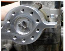
Rotate the DBW actuator and open the throttles to the fully open position using the marks previously located on the TPS housing.
