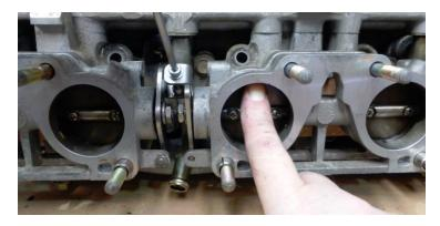
Connect the ball joint to the link arm on throttle chamber 2 and assemble the link arm as shown.
