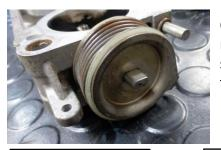
On throttle chamber 3, remove the nut and spring washer retaining the spring assembly.
