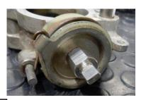
Apply some thread lock to the TPS shaft supplied and screw onto throttle chamber 3.
