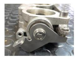
On throttle chamber 1, leave the spring arrangement on the outside. On the other side of throttle chamber 1, remove the existing link arm and attach the new link arm supplied using the existing nut and spring washer.
