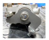
On the other side of throttle chamber 2, remove the existing link arm and attach the new link arm supplied using the existing nut and spring washer.
