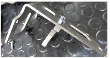
Attach the DBW support bracket to the main DBW bracket using M5 x 12 screws plus lock washers.
