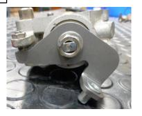
On the other side of throttle chamber 3, remove the existing link arm and attach the new link arm supplied using the existing nut and spring washer.
