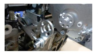
Attach the arm of the DBW lever to the rod eye on the link arm using an M5 x 16 screw and flat washer.
