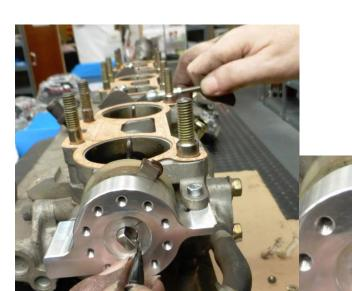
On the TPS housing mark the position of the throttle closed and throttle fully open positions. Once the intake manifold is fitted, it will not be possible to know the fully open position of the throttle blades. The closed position stops on each throttle chamber should now be adjusted if necessary.
