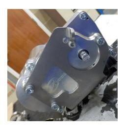
Now fit the DBW actuator onto the bracket using 3 x M5 x 10 and 1 x M4 x 10 plus washers on the outside and 2 x M5 x 16 plus washers on the inside.
