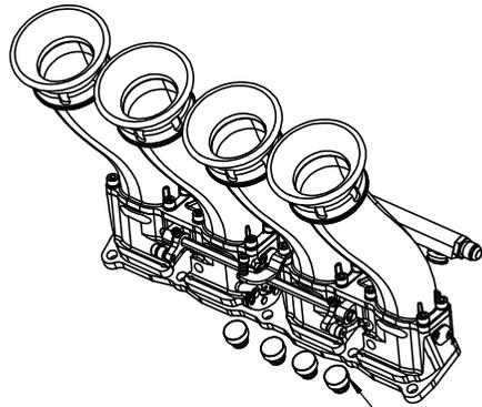
INJECTOR PLUGS FOR OEM INJECTOR
